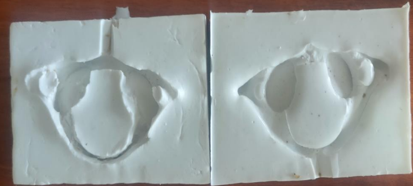
Silicon Mold of ATLAS Vertebra is prepared
